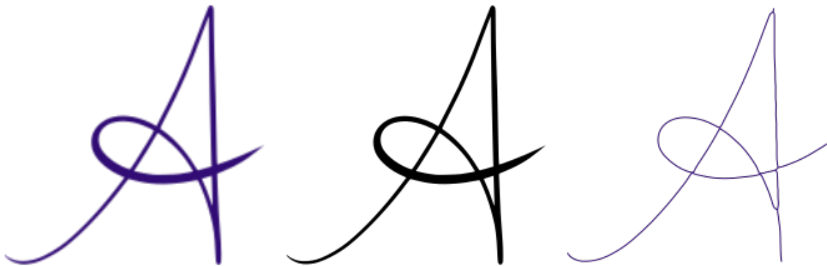
Fig. 1: The results of tracing the letter on the left with Brightness cutoff (center) and Centerline tracing (right).
