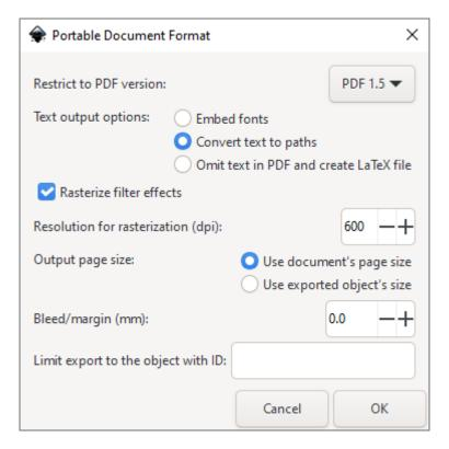
圖 1: The PDF export dialog offers many options. Usually, the default settings will work fine. However, when the PDF is for printing (as opposed to screen display), it is recommended that you set the dpi value (resolution) for filtered objects to at least 300.
