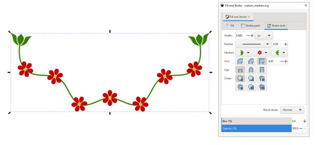
圖 3: In the Fill and Stroke dialog, we have selected the new markers for the start, end and middle of our path. They are placed on the nodes of the path. The size of the markers depends on the size of the objects that were converted to a marker. It also changes with the stroke width of the path.
